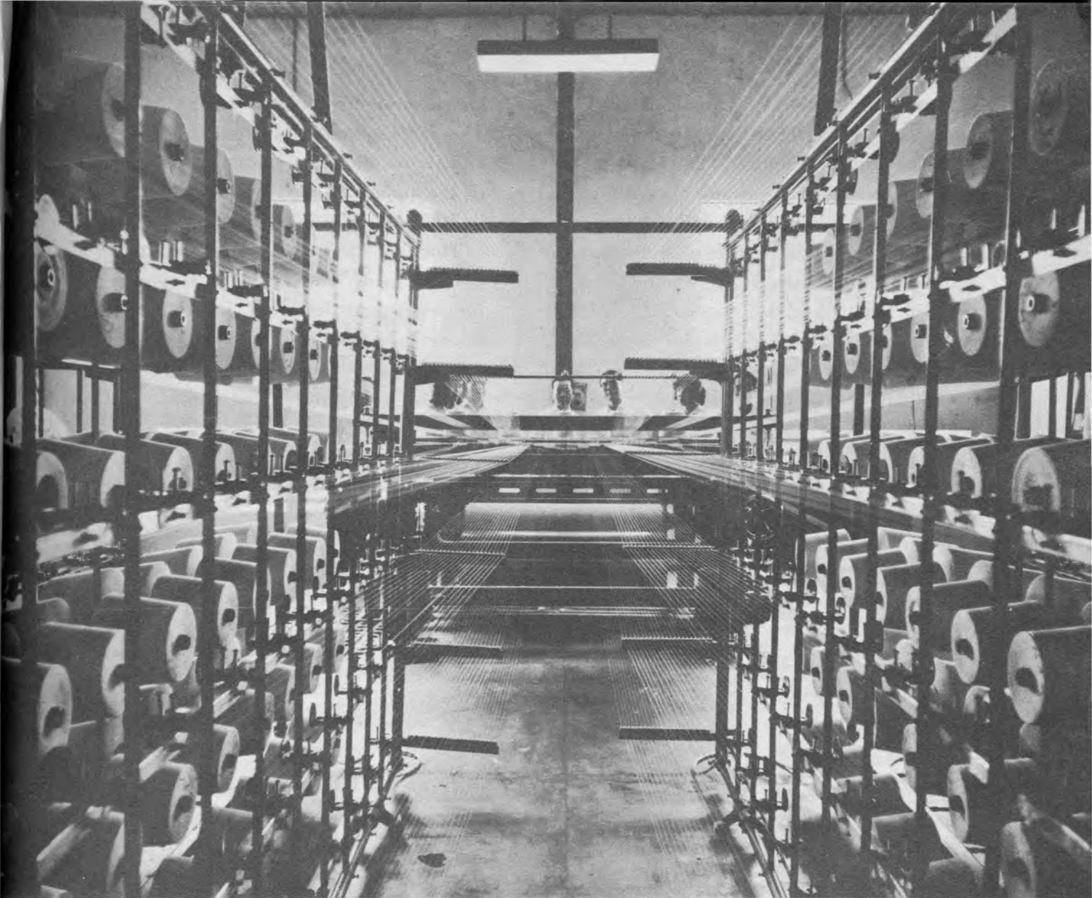
High speed warping machine installed in a large cotton fabric weaving plant.
